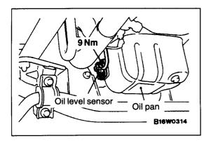
6. If there is a defect, replace the oil level sensor.
