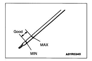
3. Pull out the level gauge slowly and check that the oil level is in the illustrated range.
