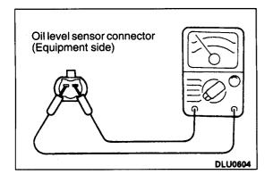
5. Check the continuity between the oil level sensor terminals.
