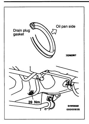
Install a new drain plug gasket so that it faces in the direction shown in the illustration, and then tighten the drain plug to the specified torque.
